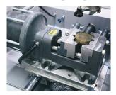
Pneumatic Clamping Device
