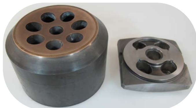
Match lapped 125mm piston pump body and swash plate
