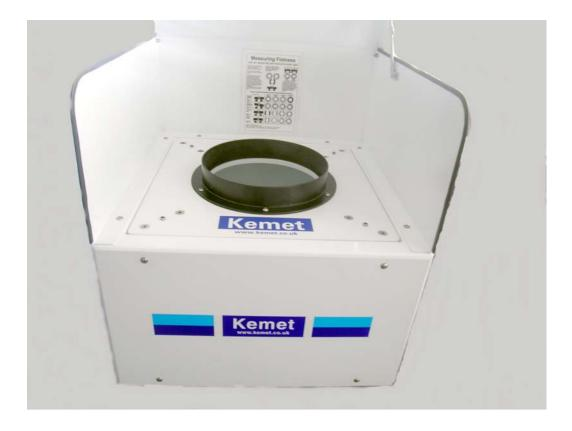
Large optical flats (Eg 250mm diameter and above) are heavy. If they are placed directly onto a thin component such as mechanical seals, they can cause distortion of the component and incorrect light band readings.
