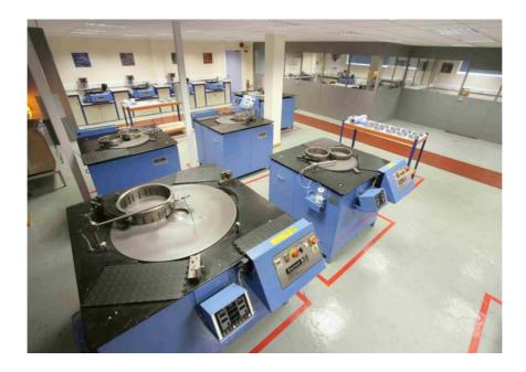
The **NEW** Flat Lapping Technical Centre is equipped with 10 Kemet Flat Lapping and Polishing Machines (15", 24", 36" diameter) along with the latest Mitutoyo Surface Measuring, Flatness Inspection Equipment and ultrasonic machines.
