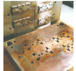
Mould before cleaning
