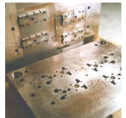
Mould after cleaning
