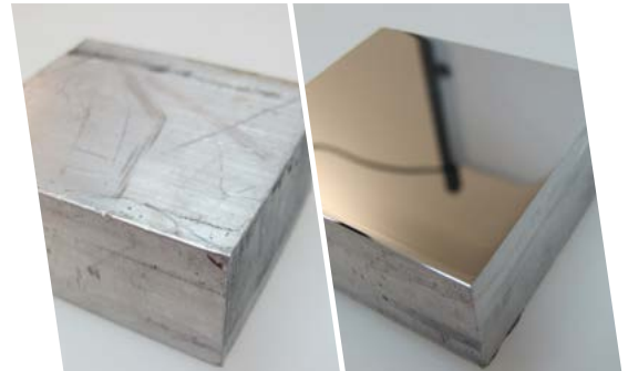
Before and after using Kemox SF on Aluminium
