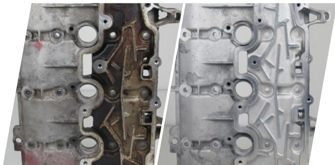
Injection Mould Plate cleaned
