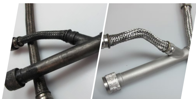
Aircraft Hydraulic Pipe Line cleaned
