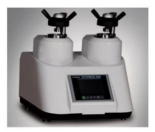
ECOPRESS 200 is an easy to use automatic hot mounting press with two cylinder. It has advanced software with programmable HMI touch screen controls. Robust bayonet closure allows for quick and safe operation. ECOPRESS offers a wide selection of mould assemblies from 25 to 50mm in diameter. Two mounts can be produced simultaneously with the use of an intermediate ram.
